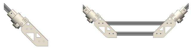
**Mobile Base**. The mobile base is consists of several European standard 30x30 / 30x60 / 60x60 aluminum profiles. Follow the provided assembly file to assemble them together.
