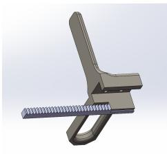
After the adhesive bonding is complete, use M3x6 screws to directly tighten the gripper fingers onto the linear guide rail's slider. The final installation result is shown as follows.
