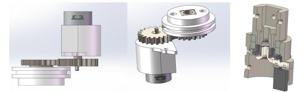
The encoder is driven by gears. The square-shaft gear fits into the square hole on the lower part of the rotating shaft. After securing the encoder to its mounting bracket, another gear is installed onto the rotating shaft. Finally, both components are assembled into the housing to achieve transmission.
