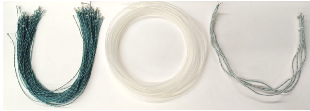
Fig. B-1. (left) 0.8mm 4-pin terminal wire; (middle) 4mm 4x heat shrink tubes; (right) wrapped wires.
